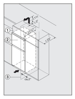
The air intake and outlet must not be blocked or covered in any way. They also need to be dusted/cleaned on a regular basis.
